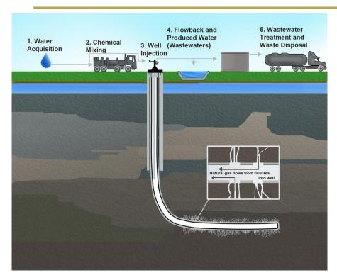
'Illustration of hydraulic fracturing and related activities', 28 February 2012, US Environmental Protection Agency, CC-PD-Mark 1.0, <a href="http://www2.epa.gov/hfstudy/hydraulic-fracturing-water-cycle">http://www2.epa.gov/hfstudy/hydraulic-fracturing-water-cycle</a>
